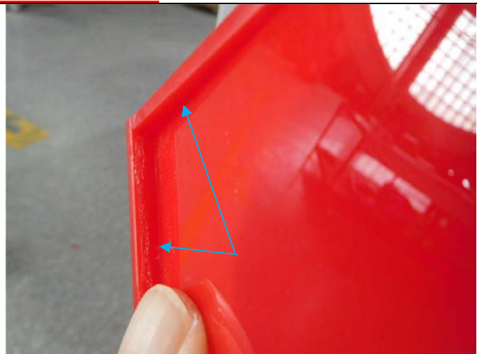
The bottom of the tray is loosed (the glue is not firmly attached)
